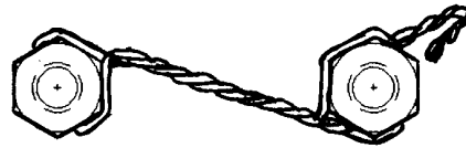
Fig 5. Typical wire locking detail
