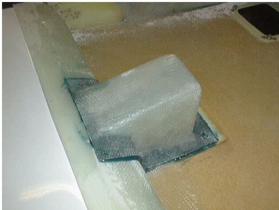
Fig 22. Aileron mass balance box bonded into place.
