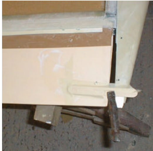
Fig 23. Aileron clamped in neutral.
