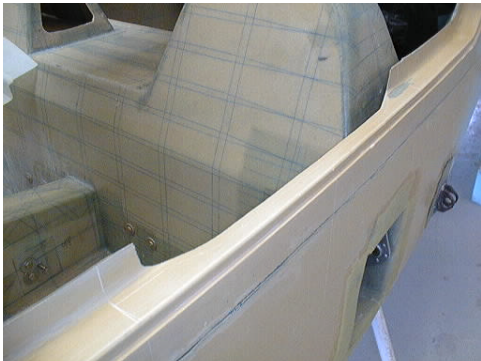
Fig 6. Photo of cut away flange.
