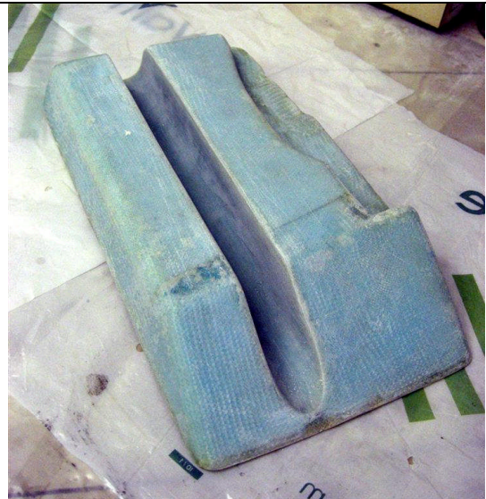
Picture 4 Push rod cover incorporated in seat base.
