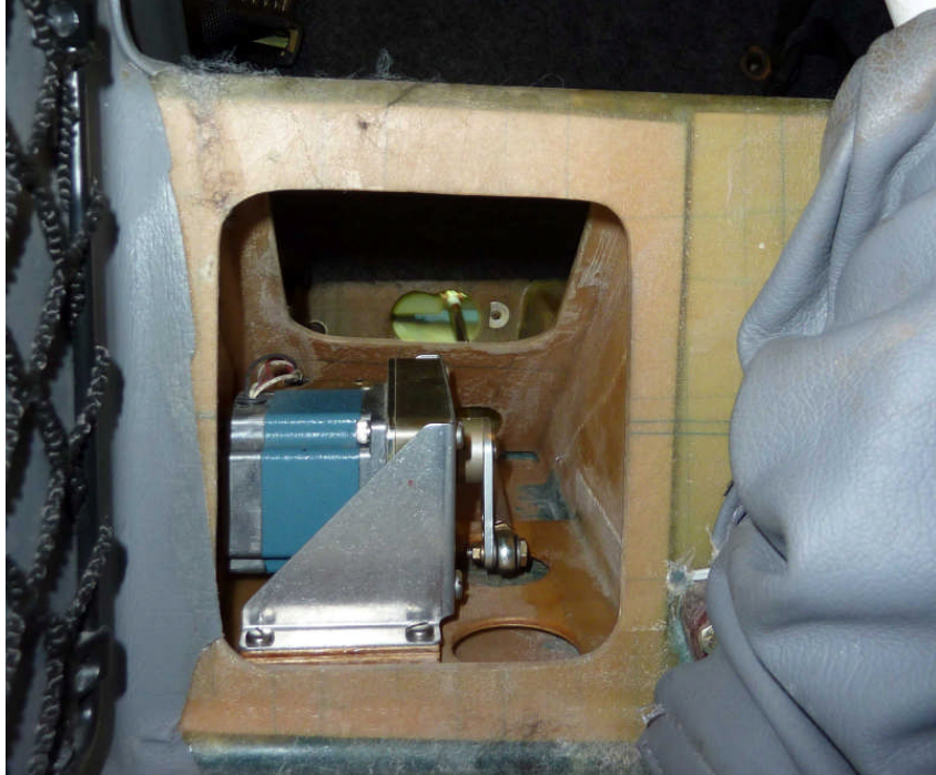
Picture 2 Example TruTrak installation. Looking aft through front face of thigh support.
