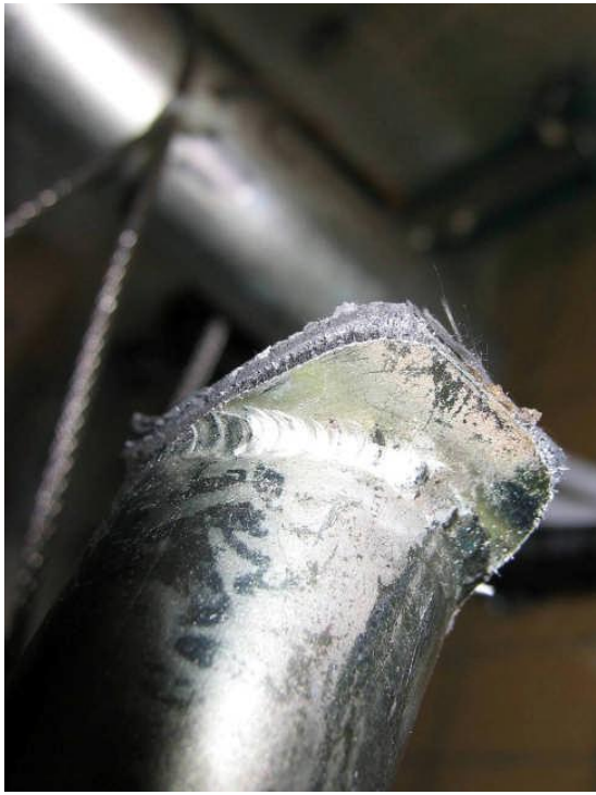
Fig 4. Bump stop sides trimmed
