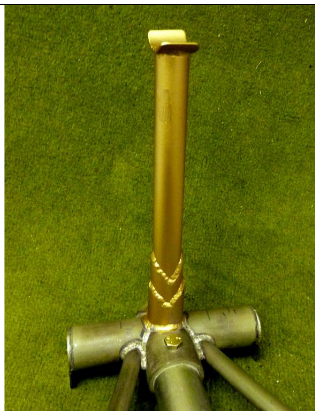
Picture 3 Reworked stop tube
