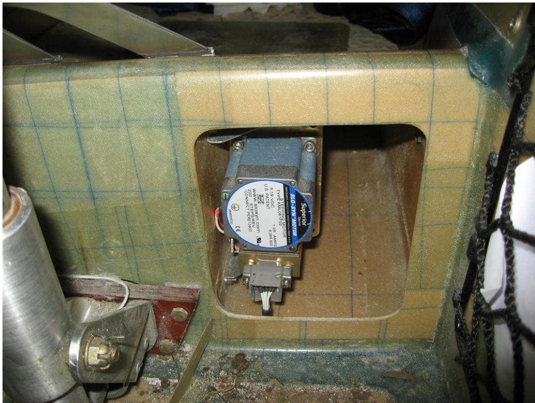
Picture 2 Example TruTrak installation. Looking aft through front face of thigh support.
