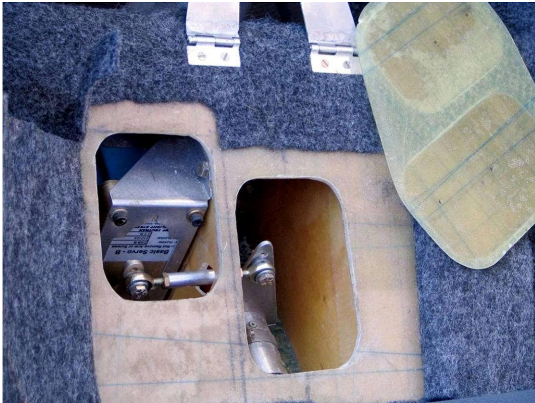
Picture 1 Example TruTrak installation. Looking down through access holes in thigh support.
