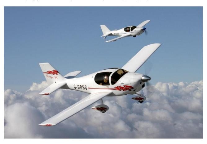
The Europa NG is a development of the Europa XS. The Europa NG differs from the XS by the introduction of pre-moulded flaps, ailerons, rudder and tailplanes and tabs. To provide cross fleet upgrades the NG tailplanes, tabs and rudder can be incorporated into a Classic and all NG pre-moulded parts could be incorporated into an XS and vice-versa.
